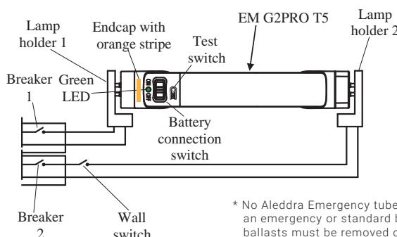
\* No Aleddra Emergency tubes can be used with an emergency or standard ballasts. The existing ballasts must be removed or by-passed.
